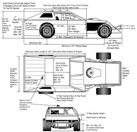
78" Maximum Body Width At Bottom Of Panels Near The Ground. You Are Not Allowed To "Flare" Bottom Edges Of Panels And Exceed Maximum Measurement Shown.
