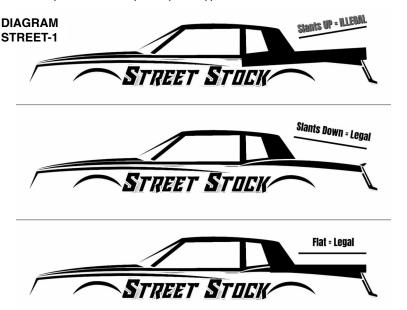
spoiler must attach to the trunk or rear quarter panels no more than 3 inches from the back of the car. The spoiler may be up to 3 inches in material, may only be as wide as the rear deck/trunk of the car, and must be straight side-to-side. Spoiler can be made of steel, aluminum or lexan. No part of the tail piece which encloses the back of the car can be above the trunk lid line. Cars equipped with the Concept Engine are not permitted to have a spoiler.
